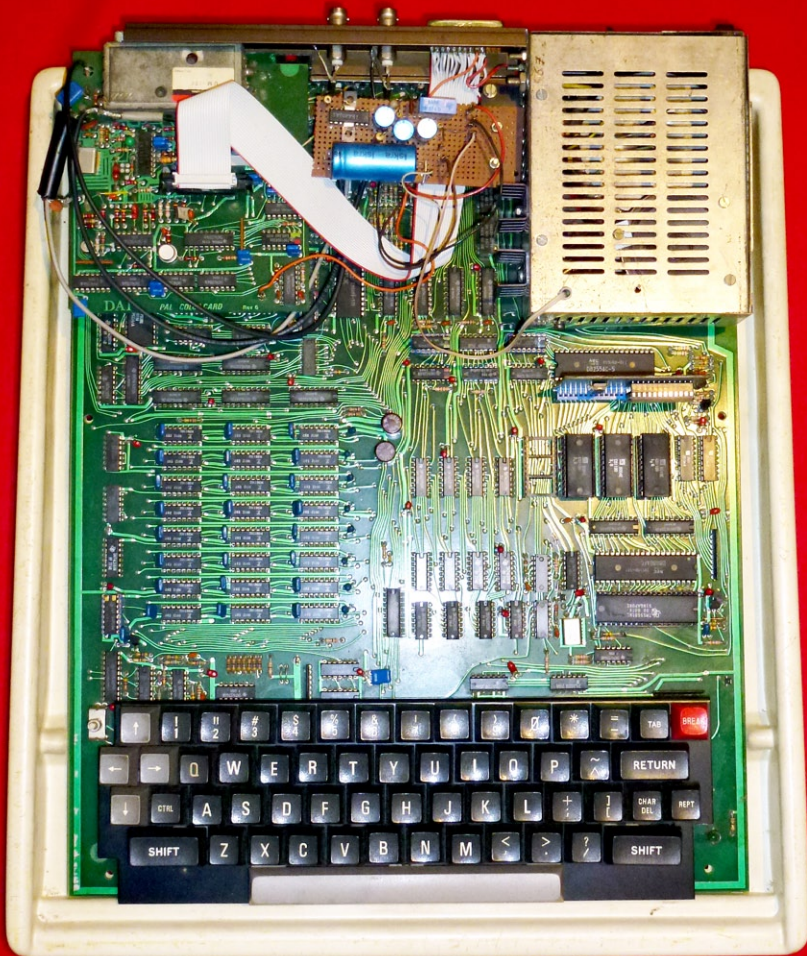
Video output modification - Model 1980
